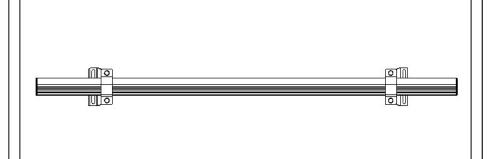
Once in position, tighten all fixings to **8Nm**. Periodically check all fixings.
